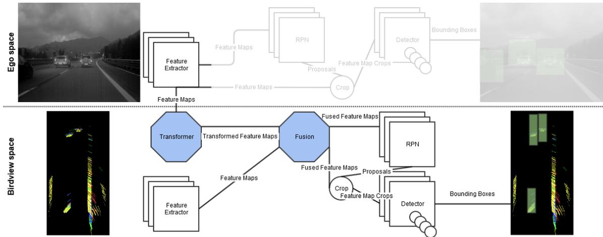
Abbildung 2: Our proposed fusion architecture. White elements denote parts of the network belonging to an arbitrary state-of-the-art object detector (Faster-RCNN [7] in our case). Blue elements denote our transformer and fusion modules mapping feature maps from ego- to birdview. This allows using camera features in addition to Lidar for predicting objects’ locations and classes. The camera-only detector is used only for training the feature extractor and can be removed afterwards.
