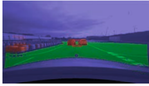
(a) Track (red box) project into labeled image (blue - background, green - road, red - vehicle)
