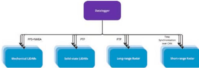
Figure 3: Overview of the created time synchronization framework
