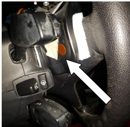
Figure 2: Implemented pressure sensor on the back of a gear shift paddle [8].
