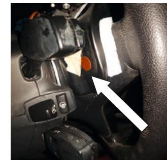
Figure 2: Implemented pressure sensor on the back of a gear shift paddle [8].
